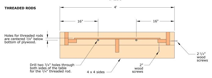
Countersink the holes  $1\,^1/^2$  dia x 1" deep on both sides of the table for the nuts and washers.
