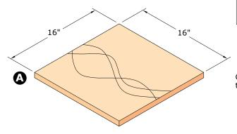
Cut the wood to size and then trace the pattern onto the wood surface.
