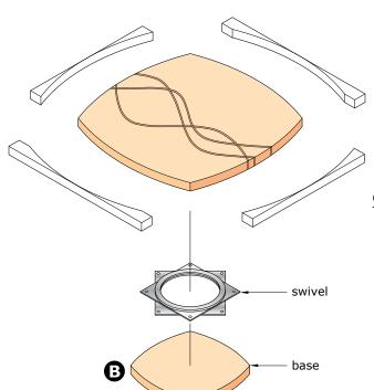
Cut arcs into the four sides. Then assemble top, swivel and base.
