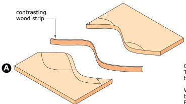
Cut through one of the pattern lines. Then glue the contrasting strip between the two top pieces.
