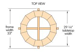
Confirm that the frame crossbars ("C" pieces) are 1/8" to 1/4" larger than the tabletop width (from flat to flat). This will allow you to place the tabletop into the frame and remove it with ease.
